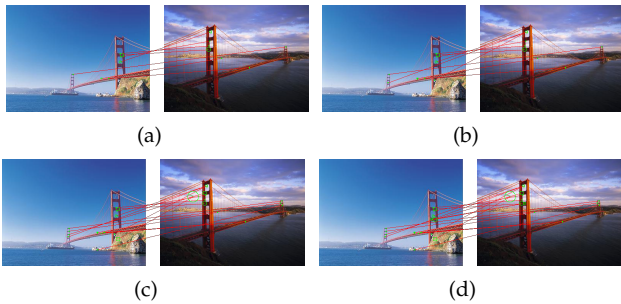
Fig. 7. (a) Result of image matching on the scheme of Hsu et al. [14], (b) Result of image matching on the scheme of Hu et al. [25], (c) Result of image matching based on our scheme, and (d) Result of image matching based on original SIFT algorithm [12].
