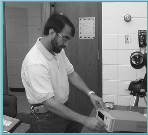
Muhammad Dawood , research assistant professor, adjusts an optical power meter to measure the laser power received through a telescope. He is conducting experiments to improve the coupling efficiency between the telescope and fiber-optic cable for an upcoming Radar Systems and Remote Sensing Laboratory (RSL) research proposal.
