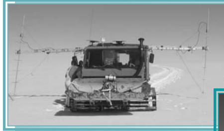
(Above) Torry Akins works with the depth sounder radar. This equipment measures surface ice thickness and maps deeper layers to help scientists determine polar ice flow and its history.
