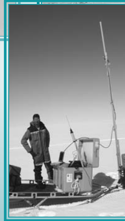
(Above) Torry Akins works with the depth sounder radar. This equipment measures surface ice thickness and maps deeper layers to help scientists determine polar ice flow and its history.
