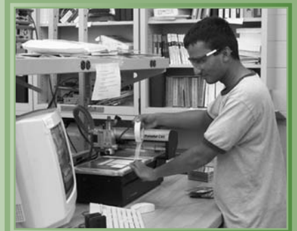
NASA Fellow Vijaya Ramasami makes a circuit board using a PCV milling machine. Currently, Ramasami is one of three NASA Fellows at the Center.
