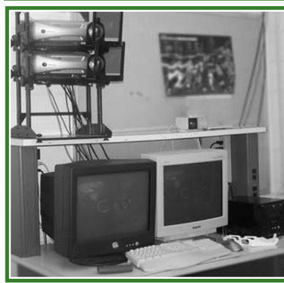
Seniors Rory Petty and Ted Weidling built GeoWall for the School of Engineering's annual Engineering Expo. The projectors, which needed special lens configurations and alignments, sit on the ledge above the computers. The computers house the content for the 3-D presentation, including a view of downtown Lawrence.
