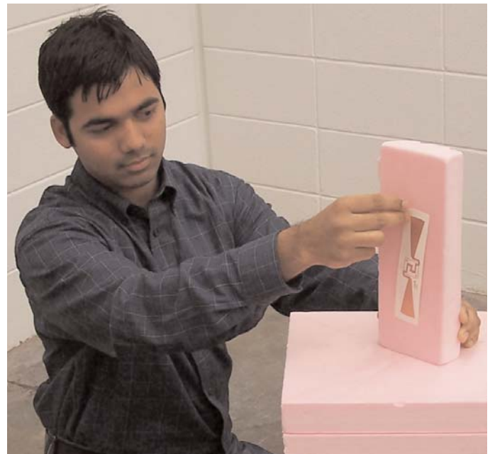
Graduate student Afzal Syed holds an RFID tag against Styrofoam in preparation for a test. Syed and other ITTC researchers have conducted numerous performance tests on various configurations of RFID tags in the RFID Alliance Laboratory.
