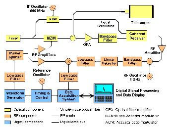
Figure 1. Block diagram of the hybrid RF/laser radar with linear detection.
