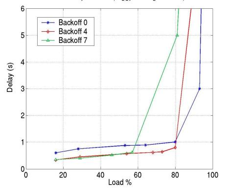
Delay vs Load (Piggybacking enabled)
