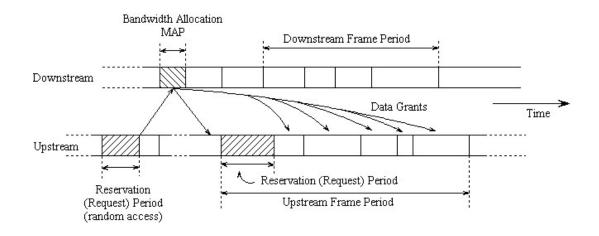
Fig. 1 Allocation MAP Structure
