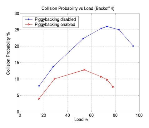
Fig. 13 Effect of Piggybacking on Collision Probability
