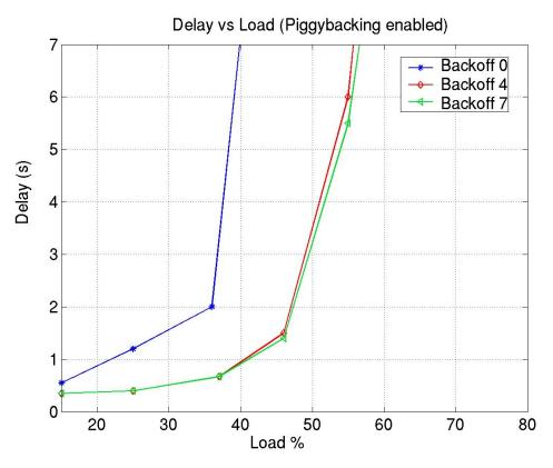
Fig. 12 Effect of Back-off on Delay (Piggybacking enabled)
