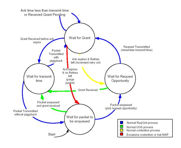
Fig. 2 State Diagram of Request/Grant Process
