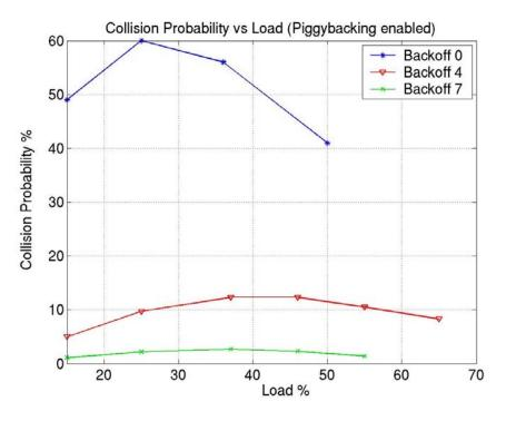
Fig. 11 Effect of Back-off on Collision Probability (Piggybacking enabled) Analysis:
