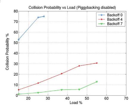
Fig. 10 Effect of Back-off on Collision Probability (Piggybacking disabled) Analysis:
