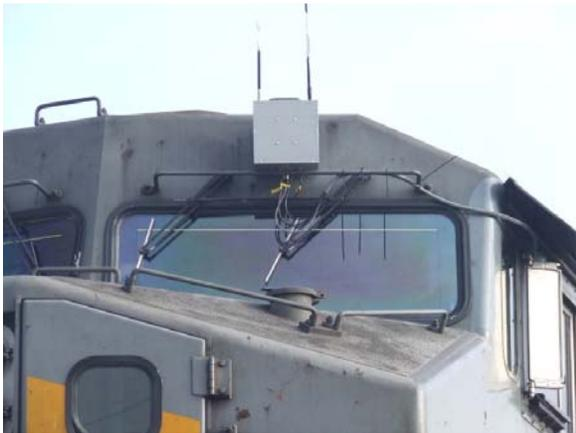
**Figure 4: Electronics box outside of locomotive during long haul test.**
