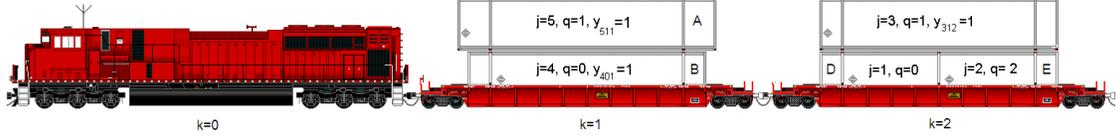
Fig. 2. Two Well-cars with Load Indices Identified
