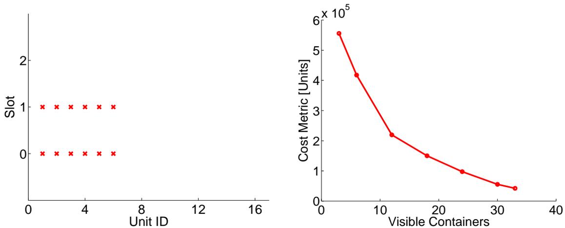
(a) Sensor Locations, where Locomotive = Unit 0, slot 0 is in the bottom level of the railcar, and slot 1 is in the top level.
