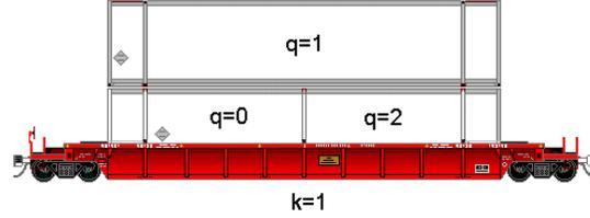
Fig. 1. Unit with Two 20 ft. Containers and One 40 ft. Container
