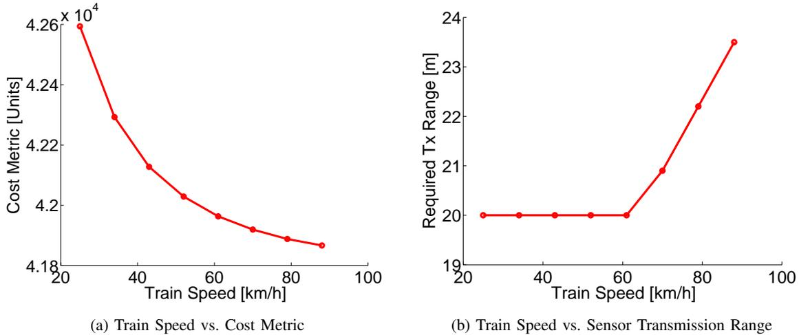
Fig. 10. Trackside Model: Train Speed versus Cost Metric and Sensor Transmission Range
