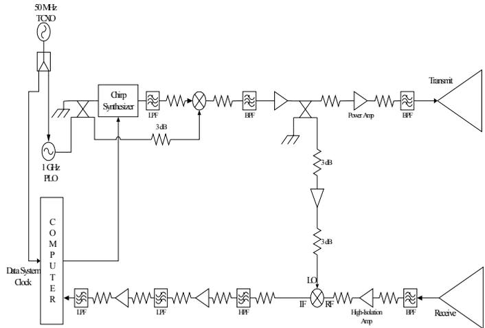
Fig. 2. Block diagram of the wideband FMCW radar system for airborne mapping of internal layers.
