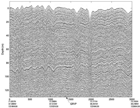
Fig. 1. Internal layers observed at the GRIP camp which is located in the dry snow region of the Greenland ice sheet.
