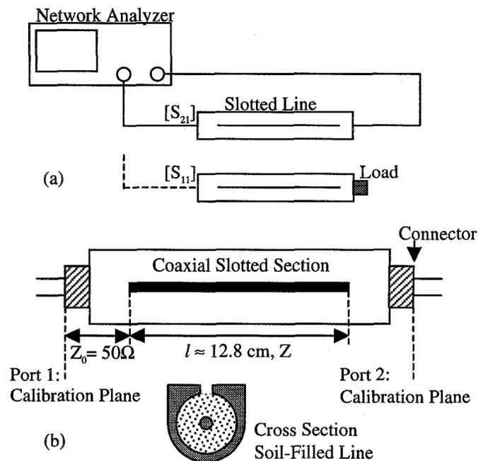
Fig. 1. (a) Configuration for either through  $[S_{21}]$  or reflection,  $[S_{11}]$  measurements. (b) Coaxial slotted section of transmission line with cross-sectional view.
