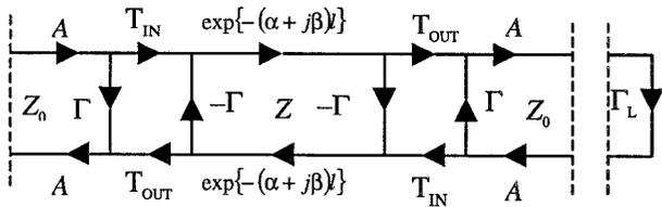
Fig. 2. Signal flow graph representation of the slotted line for the calculation of the analytical values.
