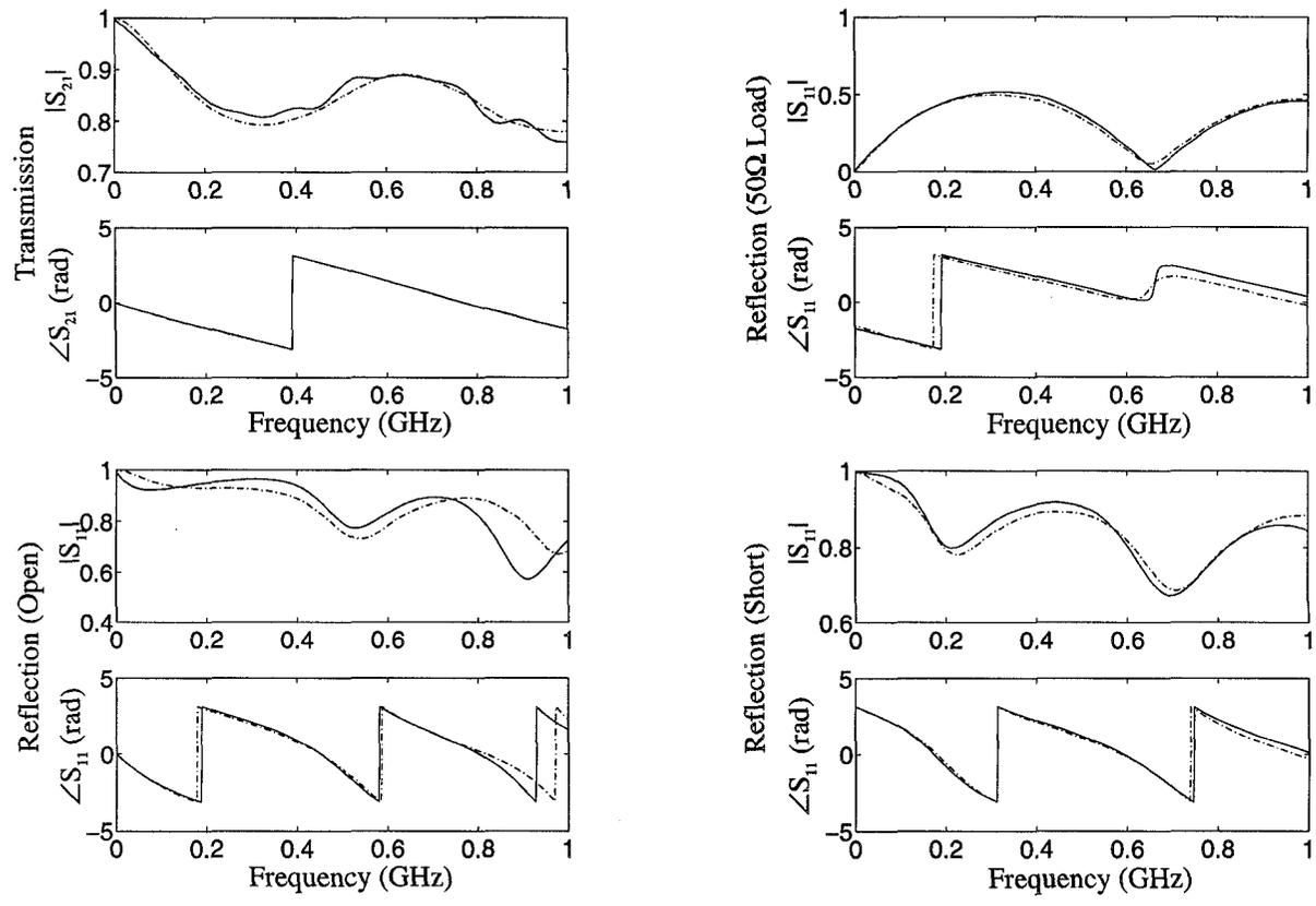
Fig. 3. Comparison of the measured (solid lines) and calculated (dashed lines) S-parameters using the soil model in Table 1.
