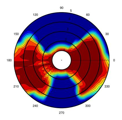
Figure 48: Rafsec on Nokia 8265 performance vs. distance and orientation in H-plane.
