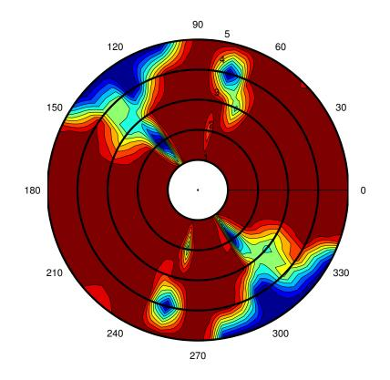
Figure 37: Alien performance vs. distance and orientation in E-plane.
