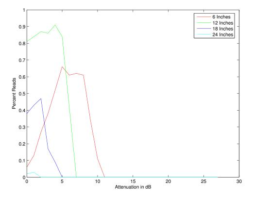
Figure 23: Avery response rate vs. distance, unmatched.
