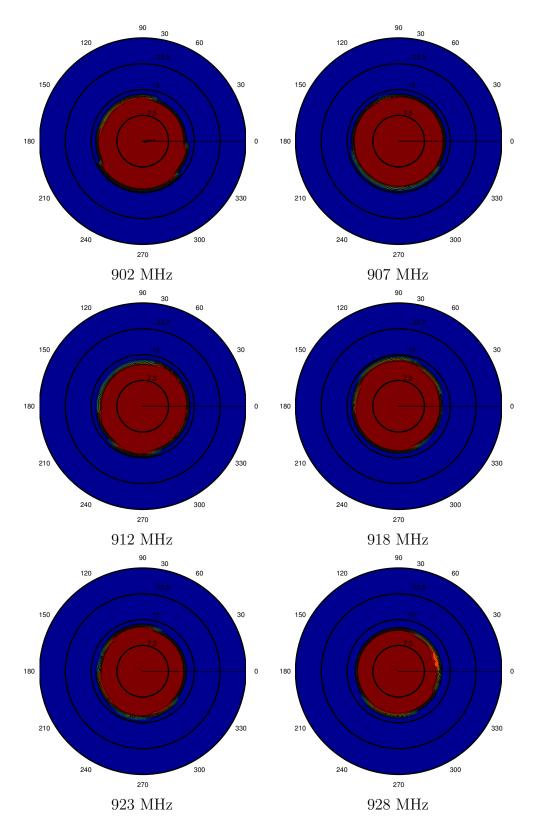
Figure 34: Radiation pattern of Rafsec tag in H-plane, matched configuration.
