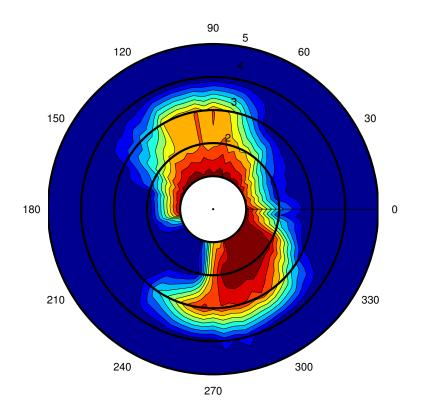
Figure 40: Avery performance vs. distance and orientation in H-plane.
