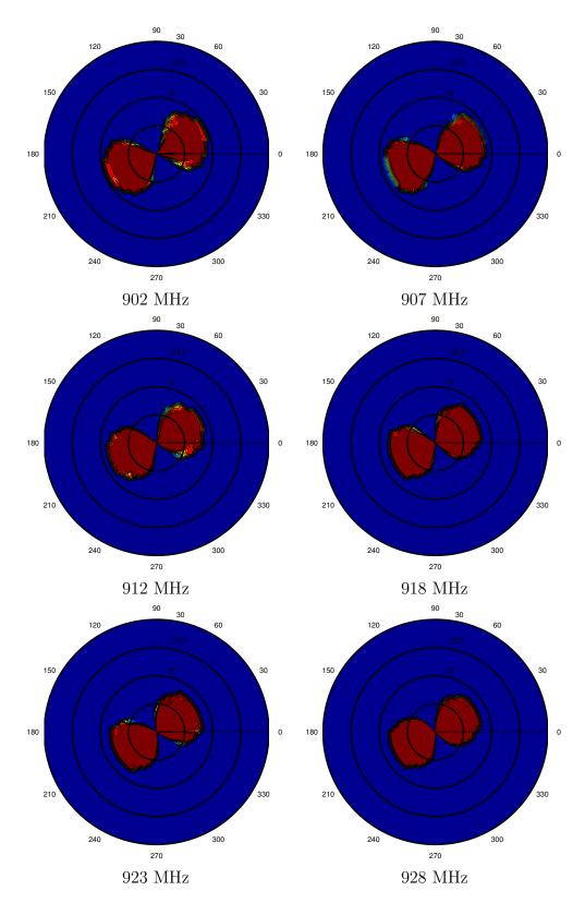
Figure 33: Radiation pattern of Rafsec tag in E-plane, unmatched configuration.
