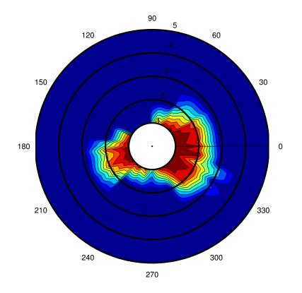
Figure 54: Rafsec on Sony T610 performance vs. distance and orientation in H-plane.
