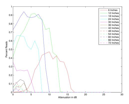
Figure 24: Rafsec response rate vs. distance, unmatched.
