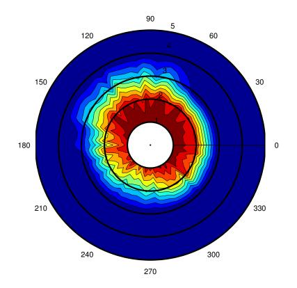
Figure 53: Rafsec on Sony T610 performance vs. distance and orientation in E-plane.
