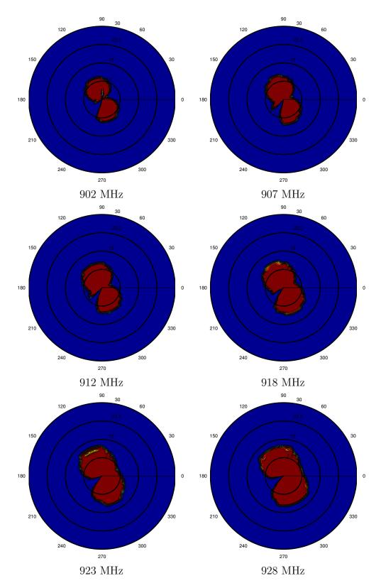
Figure 32: Radiation pattern of Avery tag in H-plane, matched configuration.
