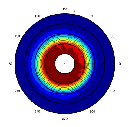
Figure 44: Symbol performance vs. distance and orientation in H-plane.
