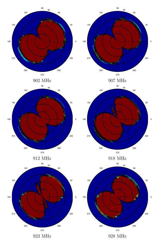
Figure 29: Radiation pattern of Alien tag in E-plane, unmatched configuration.
