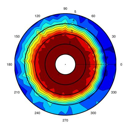
Figure 42: Rafsec performance vs. distance and orientation in H-plane.
