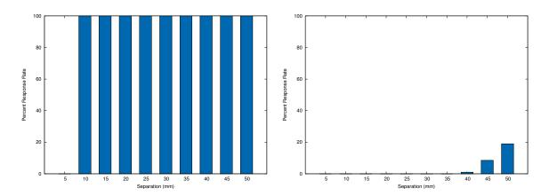
Figure 59: Alien response rate near metal. Figure 60: Avery response rate near metal.
