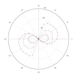
Figure 26: Minimum power level vs. orientation for three tag placements.
