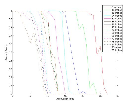
Figure 22: Alien response rate vs. distance, unmatched.
