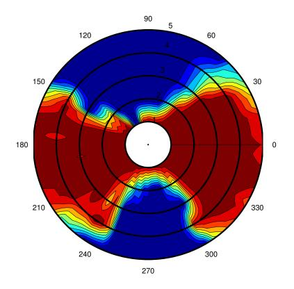
Figure 50: Rafsec on Nokia 3560 performance vs. distance and orientation in H-plane.
