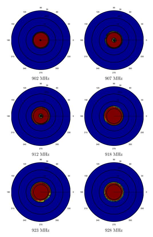
Figure 36: Radiation pattern of Symbol tag in H-plane, matched configuration.
