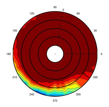
Figure 49: Rafsec on Nokia 3560 performance vs. distance and orientation in E-plane.
