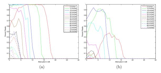
Figure 7: Rafsec tag response rate vs. distance and power: (a) matched orientation, and (b) unmatched orientation.
