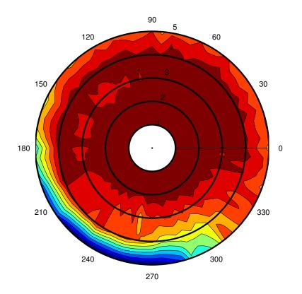
Figure 51: Rafsec on Nokia 63401 performance vs. distance and orientation in E-plane.
