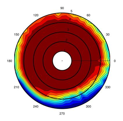
Figure 45: Rafsec on Nokia 3360 performance vs. distance and orientation in E-plane.
