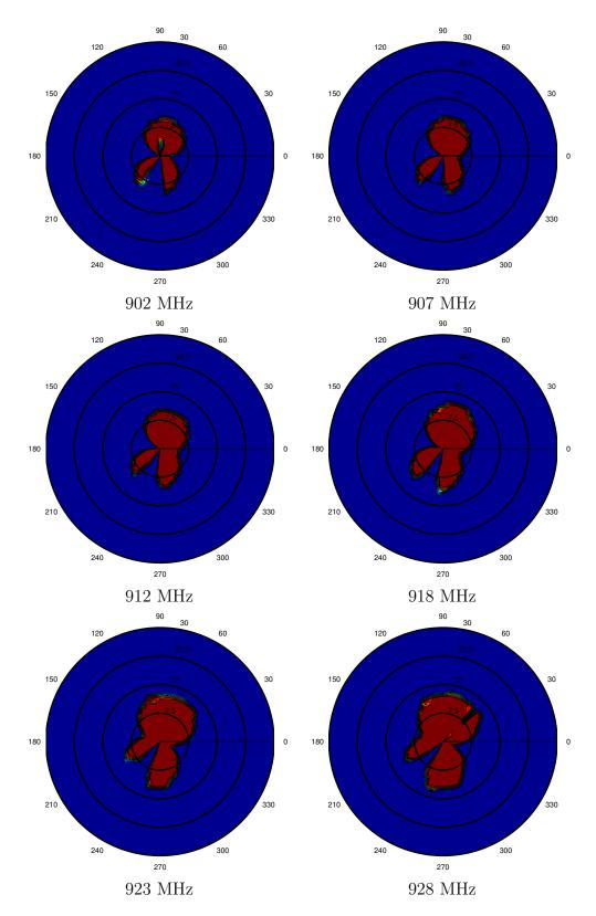
Figure 31: Radiation pattern of Avery tag in E-plane, unmatched configuration.
