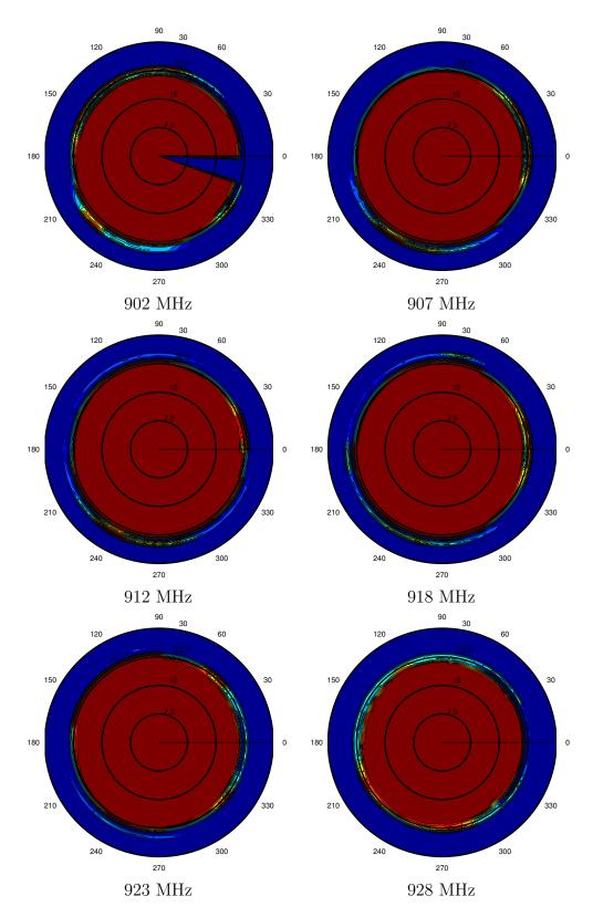
Figure 30: Radiation pattern of Alien tag in H-plane, matched configuration.
