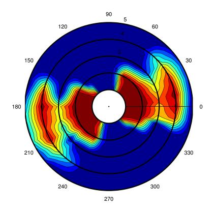
Figure 41: Rafsec performance vs. distance and orientation in E-plane.
