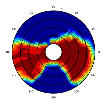
Figure 46: Rafsec on Nokia 3360 performance vs. distance and orientation in H-plane.
