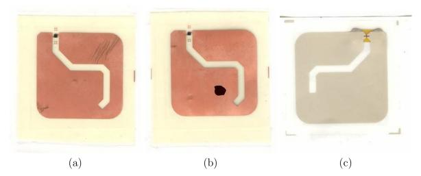
Figure 2: Avery Dennison item-level tags: (a) Avery Dennison AD-010 inlay, good (this is the tag we tested in this report) (b) Avery Dennison AD-010 inlay, marked bad, and (c) slightly older Avery Dennison AD-010 sample utilizing a strap and slightly different antenna.
