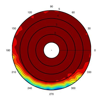
Figure 47: Rafsec on Nokia 8265 performance vs. distance and orientation in E-plane.
