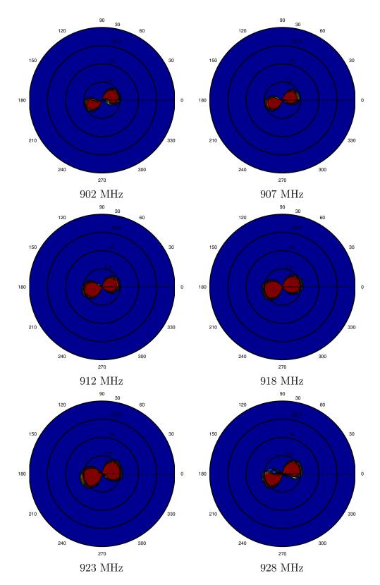
Figure 35: Radiation pattern of Symbol tag in E-plane, unmatched configuration.
