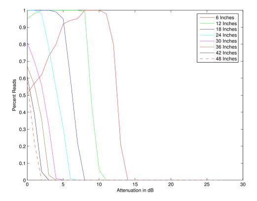
Figure 25: Symbol response rate vs. distance, unmatched.
