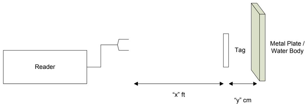
**Figure 19 Test setup for performance in front of materials**
