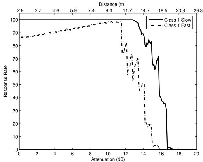
**Figure 8 Class 1 Slow vs. Fast Response rate Behavior**
