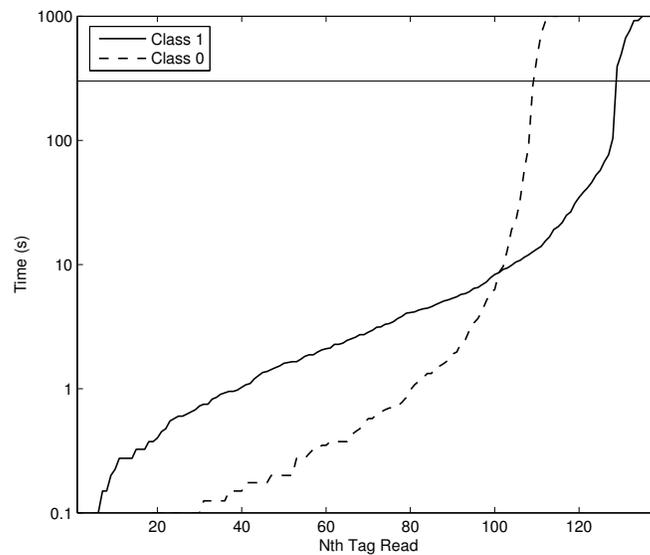
**Figure 17 Time to First Read (TTFR) for Class 0 and Class 1**
