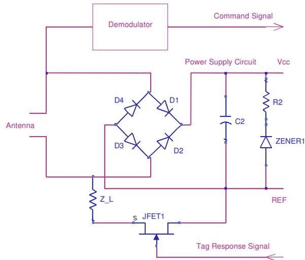
**Figure 5 Part of the circuit for a RFID tag**
