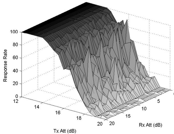
**Figure 26 Channel Sensitivity for Large tags**
