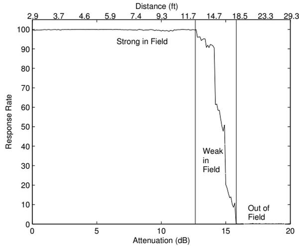
**Figure 7 Typical Response rate vs. Attenuation for a tag**
