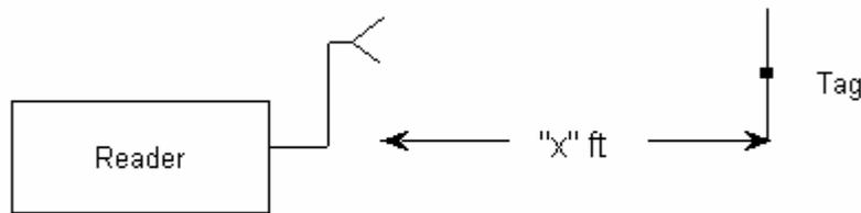
**Figure 6 Free Space experimental Setup**
