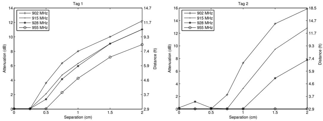
**Figure 22 Comparison of tags in front of metal based on Frequency**
