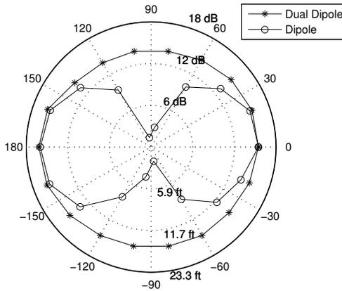
**Figure 10 Orientation Sensitivity of Two tags along E-plane**
