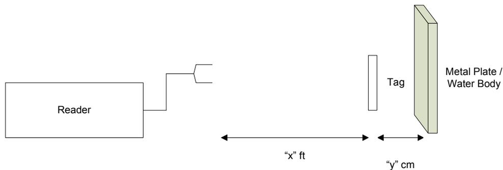
**Figure 19 Test setup for performance in front of materials**
