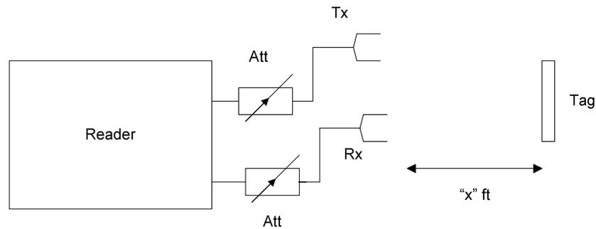
**Figure 25 Test setup for channel sensitivity**
