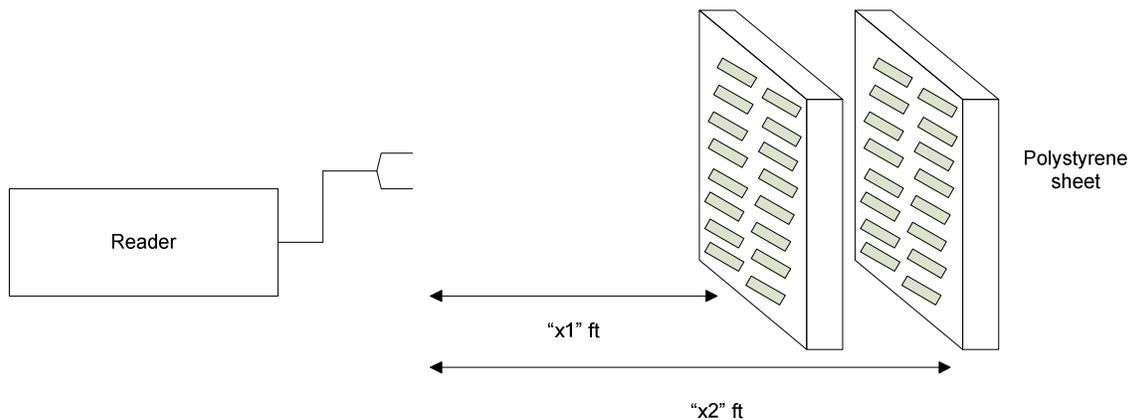
Figure 15 Class 0 tags and Class 1 tags setup for read rates in population experiment
