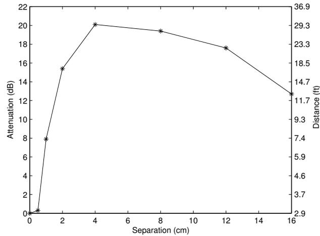
**Figure 31 Better Performance of a tag in front of metal**
