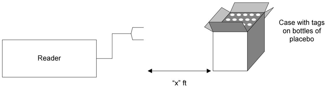
**Figure 16 Class 0 item-level tags setup for read rates in population experiment**
