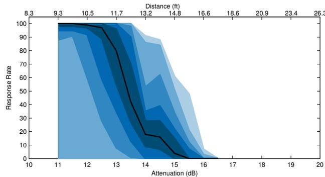
**Figure 12 Typical variance of performance among tested commercial tag models**
