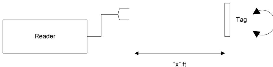
**Figure 9 Test setup for orientation sensitivity**
