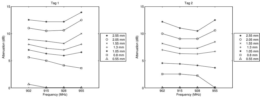
**Figure 23 Comparison of tags in front of water based on Frequency**
