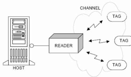
**Figure 2 RFID system components**
