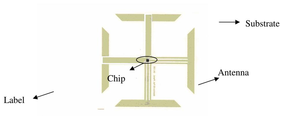
**Figure 3 Sample Passive RFID tag**
