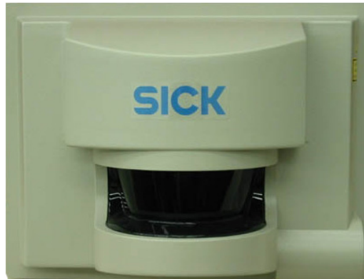
Figure 5.2: Sick LMS 221 laser range finder.
