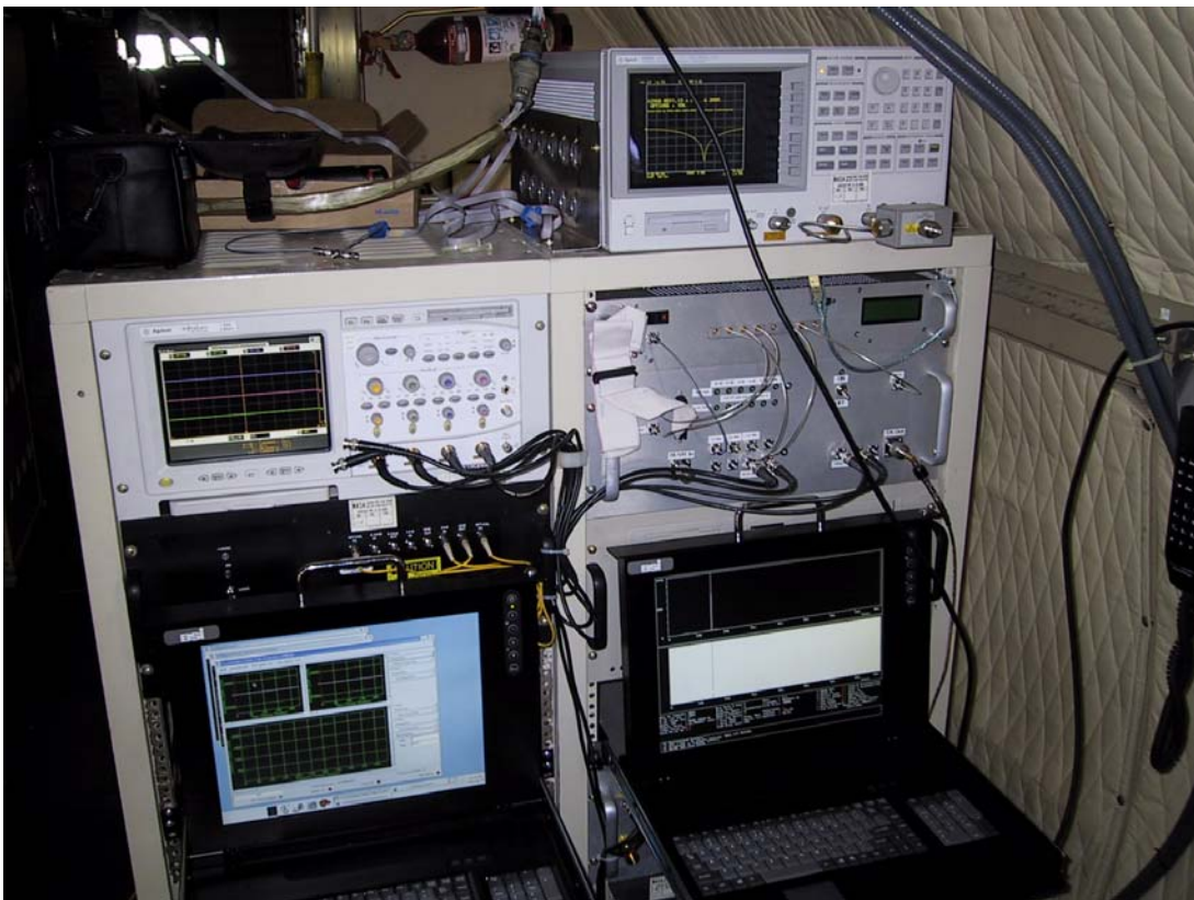
Figure 4.1: ACORDS system after mounting inside the pressurized cabin of the NASA P3 aircraft
