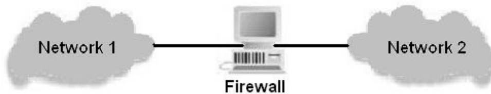
Figure 7.1: A single firewall between two networks
