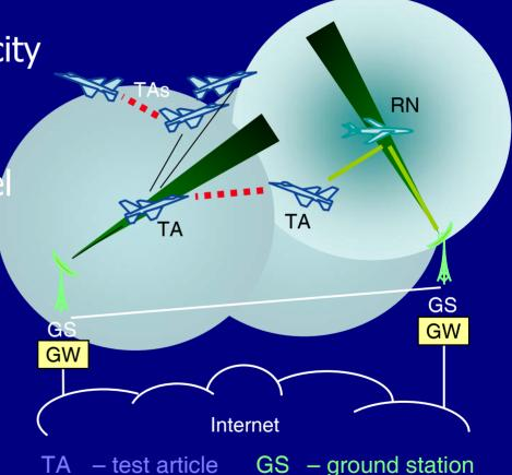
TA – test article GS – ground statior RN – relay node GW – gateway
