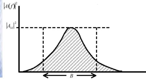
Note: Since spectral noise components are non-correlated, one must integrate over the noise power.
