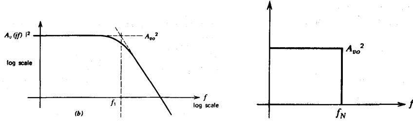
\* Frequency  $f_N$  is chosen to give the *same* total output noise voltage as the original circuit when the same input noise voltage is applied. Thus
