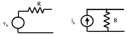
The noise contributed by the resistor is modeled by the source, thus the resistor is considered noiseless.
