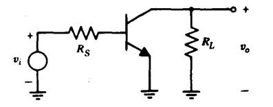
Consider the noise performance of the simple transistor stage with the ac schematic shown below
