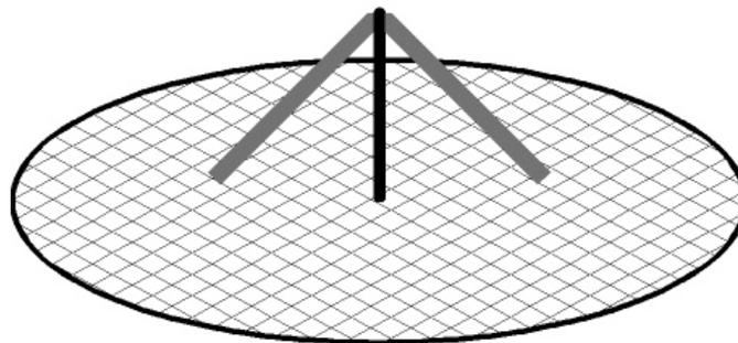
The flat reflector is still a topic of research, the idea being that it can be of limited size and extended beyond by using the ground as a reflecting surface. The small reflector would be effective at the upper frequency of operation where noise performance is critical. At lower frequencies this is not an issue and the ground might be a suitable reflector and this would lead to a cost saving.
