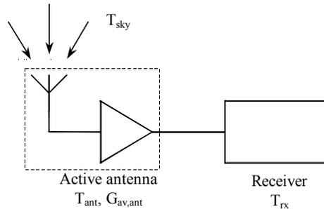
In general the noise contribution of the receiver is minimised by having a reasonable low value of  $T_{\text{rx}}$ , but more important by choosing the available gain of the active antenna sufficiently large.
