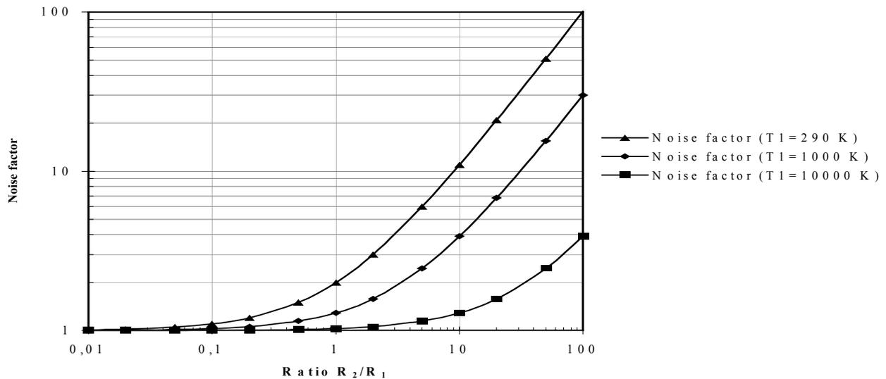
The noise in the amplifier is caused by thermal noise in dissipative elements and various sources of non-thermal noise in active components like transistors. Depending on circuit topology and used components the noise contribution of this part can normally not be neglected. Section 3.5 describes in more detail this topic and how to minimise this noise contributions.
