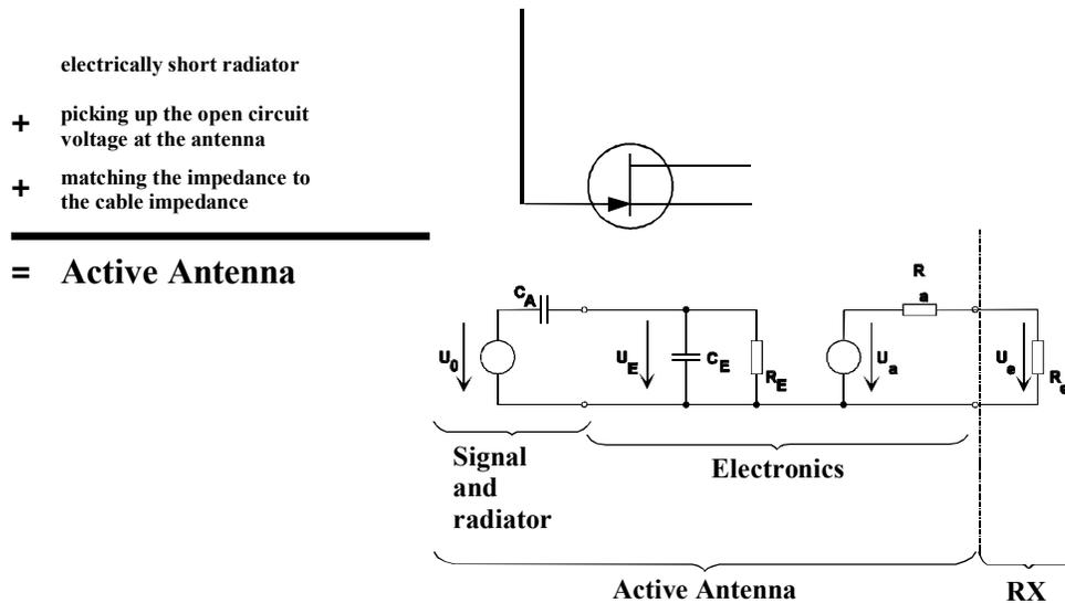
These features have meanwhile led to active antennas for higher frequencies as well. Particularly at frequencies well above 100 MHz the active device does not only transform the impedance but also amplify the signal a little bit in order to compensate cable losses. However, active antennas must never be confused with receiving systems consisting of passive antenna and antenna amplifier, and the main task for the active circuit is always the impedance transformation.
