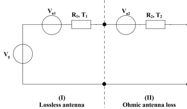
The signal degradation due to the losses can be expressed in the noise factor of a two-port that is represented by (II). The noise factor is defined as:
