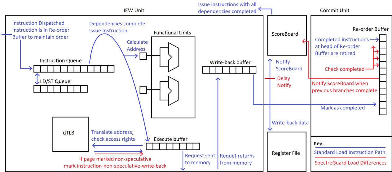
Figure 2: Micro-architectural changes needed to implement SpectreGuard.
