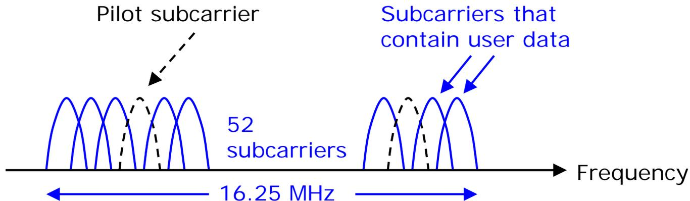
48 data subcarriers + 4 pilot subcarriers. There is a "null" at the center carrier. Around each data subcarrier is centered a subchannel carrying a low bitrate data signal (low bitrate => no intersymbol interference).
