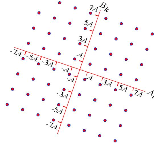
Received 64 QAM Constellation with only phase and amplitude offsets. No channel and no noise
