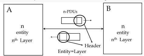
PDU stands for Protocol Data Unit, which is the data unit that is created at each layer of the network stack.
