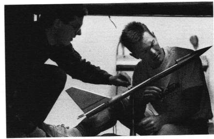
Aerospace Engineering graduate students install a generic fighter model in a low speed wind tunnel.
