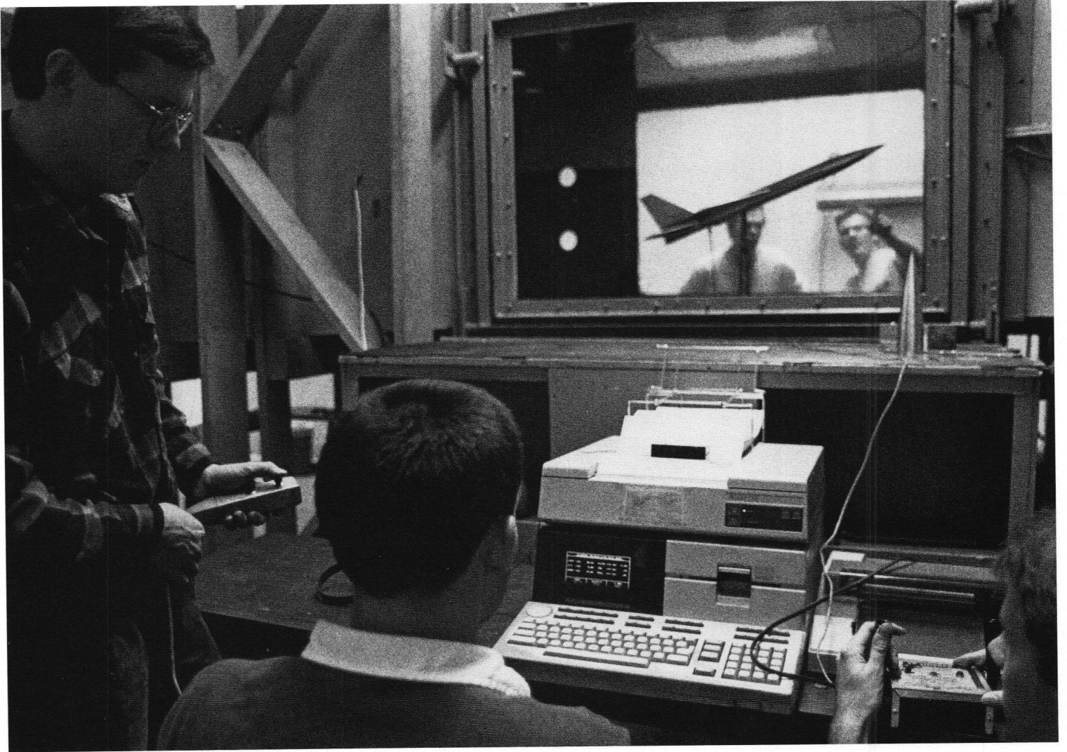
Aerospace Engineering graduate student run wind tunnel tests to determine the influence of forebody shape on vortex flow.
