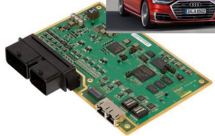
Audi's zFAS platform. 2016-2018 A single-board computer with multiple CPUs, GPU, FPGA
