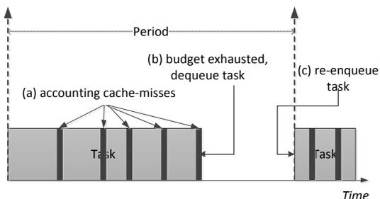
Figure 2: Basic throttling mechanism.
