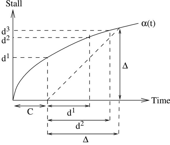
**Figure 4:** The circular dependency between the traffic from throttled core and the stall of task on the critical core,  $d$  represents the amount of traffic for a given time interval while  $\Delta$  represents the overall stall for this task.
