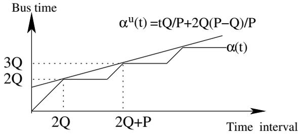
**Figure 3:** Arrival curve and its upper bound for one throttled core with  $P$  as period and  $Q$  as the cache-miss budget.
