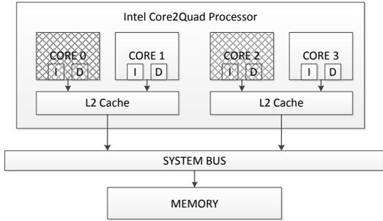
Figure 5: Architecture of our evaluation platform.
