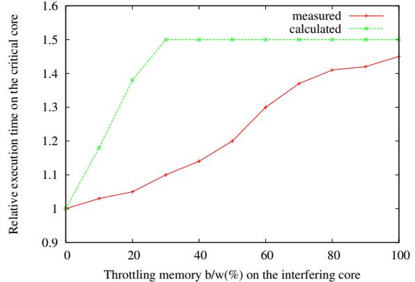
Figure 7: Impact of throttling bandwidth to the response time on the critical core.
