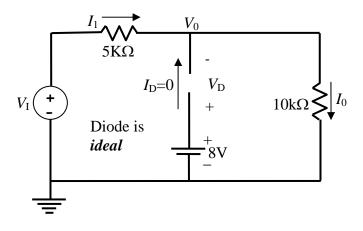
[Note: if you assume diode forward bias,  $V_0 = 8V$ ,  $I_0 = 0.8mA$ ,  $I_1 = (15V - 8V)/5k\Omega = 1.4mA$ , thus  $I_D = I_0 - I_1 = 0.8mA - 1.4mA = -0.6mA$ . Assumption is wrong.]
