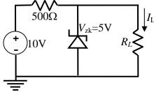
2, (30 pts) For the circuit on the right, the diode is *ideal*. For the input voltage  $V_{\rm I}$  of 15V and 10V, respectively, please analyze the circuit and find the corresponding values of  $I_0$ ,  $I_{\rm D}$  and  $V_{\rm D}$  as marked in the circuit.
