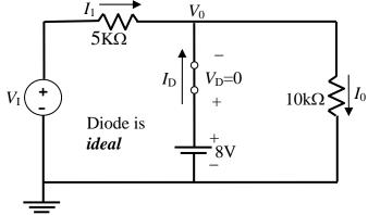
so that the current flowing through the diode is  $I_D = I_0 - I_1 = 0.8 - 0.4 = 0.4 \text{ mA} > 0$  which is positive. This verifies the forward bias assumption.
