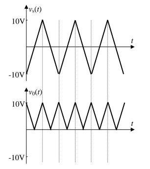
The average output voltage is  $V_{0,ave} = 5V$
