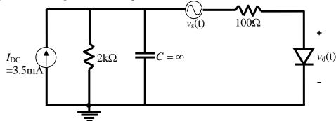
(a) Perform DC analysis and find the DC current flowing through the diode ( $I_d = ?$ )
