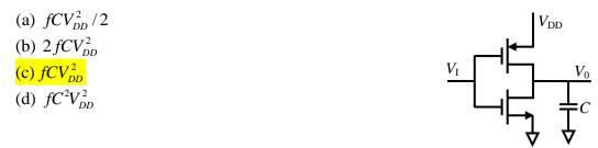
2. (30 pts.) Consider the following CMOS inverter with a bias voltage  $V_{DD} = 6V$ , the parameters of MOSFETS are: for the PMOS  $(Q_P)$ ,  $k_p = C_{ox}\mu_p(W/L) = 1mA/V^2$ ,  $V_{tp} = -1V$ , and for the NMOS  $(Q_N)$ :  $k_n = C_{ox}\mu_n(W/L) = 1mA/V^2$ ,  $V_{tm} = 1V$ .
