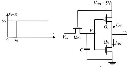
(1) Assume the NMOS transmission gate,  $Q_{N1}$ , has  $k_n = 1mA/V^2$  and  $V_t=1V$ , and the body effect can be neglected for simplicity (that is  $\gamma = 0$ ). At time t = t<sub>0</sub>, the input voltage  $V_{IN}$  is switched from 0 to 5V. Please find:
