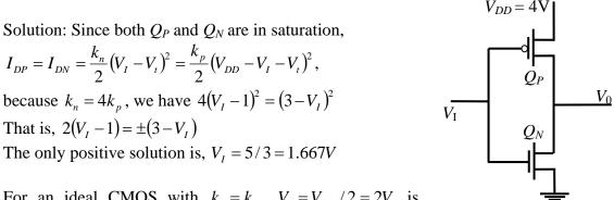
For an ideal CMOS with  $k_n = k_p$ ,  $V_I = V_{DD} / 2 = 2V$  is required to have  $V_0 = 2V$ .
