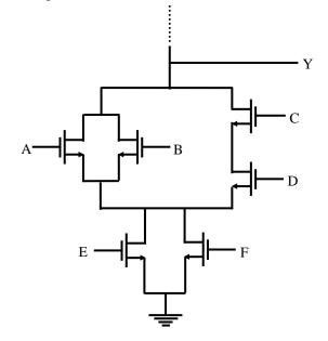
(2) (15 pts) Assume the *PUN* is a "depletion- load" based on a depletion-NMOS shown in the following circuit with parameters:  $k_n = 0.1mA/V^2$  and  $V_t = -1V$ . The bias voltage is  $V_{DD} = 3V$ .
