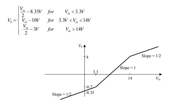
5, The circuit shown below is a diode limiter. Determine and draw the transfer characteristics ( $V_0$  versus  $V_i$ ). Be sure and label all relevant values (slope, intercept points, maximum values, etc.).
