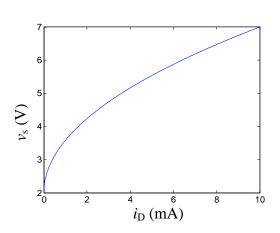
$v_{GS} = v_{DS}$ , for iD > 0, NMOS must be operate in saturation:
