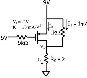
Since  $I_1 = 1mA$  is given, we can immediately find that  $V_{SD} = I_1 \cdot 1k\Omega = 1V$ , and  $V_{SG} = 9 - 5 = 4V$ . In this case,  $V_{SD} < V_{SG} - |V_t| = 4 - 2 = 2V$  the FET is in triode mode.
