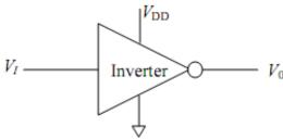
If the DC bias voltage is  $V_{DD} = 5V$ , find  $V_{IH}$ ,  $V_{IL}$ ,  $V_{0H}$ ,  $V_{0L}$ ,  $NM_L$ , and  $NM_H$ . (Use  $dV_0 / dV_L = -1$  to determine the boundary of regions).
