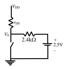
(b) When  $V_I = 5V$ , PMOS  $(Q_p)$  is cutoff and NMOS  $(Q_n)$  is triode, and the equivalent resistance of  $Q_n$  is,
