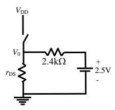
(c) When  $V_I = 2.5$ V, the output is  $V_0 = 2.5$ V due to the symmetry of the circuit. Both of the two MOSFETs are in saturation mode, and
