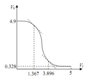
Therefore,  $V_{IL} = 1.367$ ,  $V_{IH} = 3.896$ ,  $V_{0L} = 0.328$  and  $V_{0H} = 4.9$   $NM_L = V_{IL} - V_{0L} = 1.367 - 0.328 = 1.039V$  $NM_H = V_{0H} - V_{IH} = 4.9 - 3.896 = 1.004V$  Handout problem 2:
