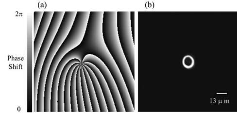
Fig. 2. (a) Phase mask employed for producing a Bessel beam with  $n = 10$  and  $r_0 = 0.8$  mm. (b) Transverse intensity distribution at the focus of lens in air. The scale bar is  $13 \mu\text{m}$ .
