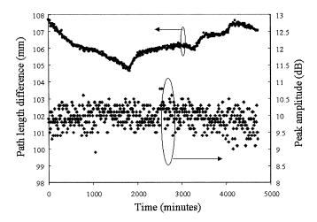
Fig. 6. Results of continuous fiber length monitoring for 5000 minutes. Dots: Measured fiber length versus time. Diamonds: Coherent interference peak amplitude versus time.
