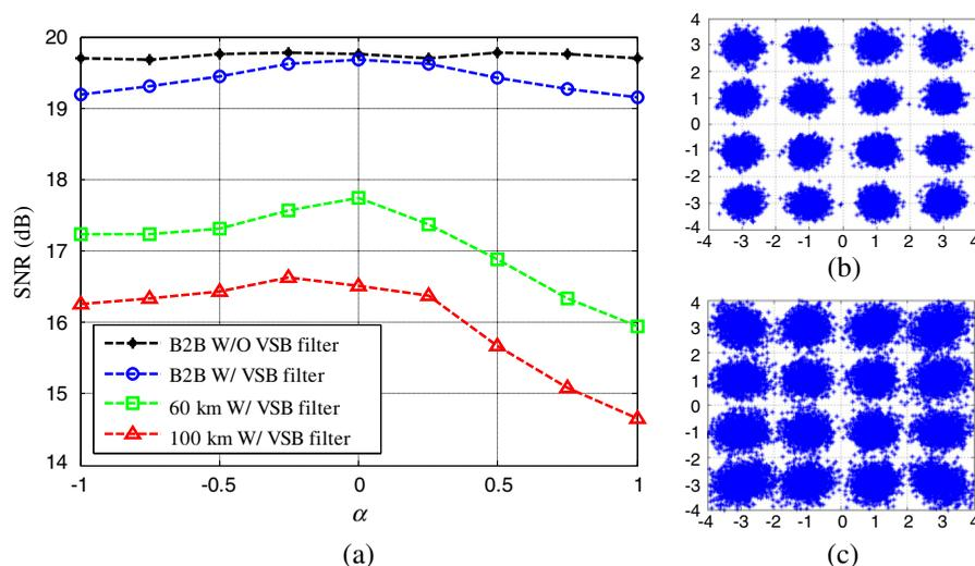
**Fig. 2** (a) Measured signal-to-noise ratio (SNR) versus chirp parameter. (b) The constellations at B2B with chirp free and without VSB filter. (c) The constellations after 100-km standard single-mode fiber transmission with chirp free and with VSB filter.
