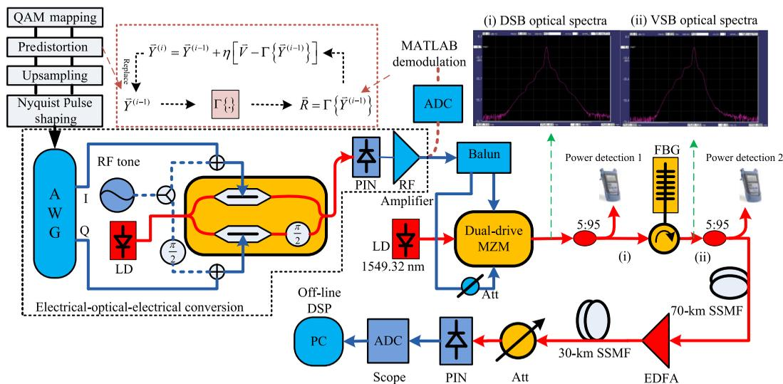
**Fig. 1** Experimental setup of fiber Bragg grating (FBG)-based vestigial sideband (VSB)-IMDD half-cycle Nyquist-subcarrier modulation (SCM) transmission system and the optical spectra (a) before and (b) after FBG filter.
