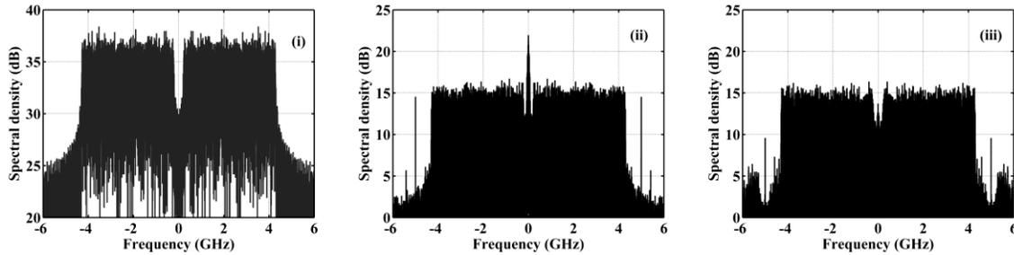
Fig. 4. OFDM spectra without 50% guard band, generated at the CO (i), measured at the CU using CER (ii) and measured at the CU using self-homodyne (iii).
