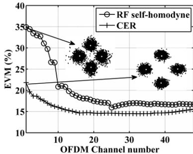
Fig. 5. Relative system performance for two RF down conversion techniques for each subcarrier. The insets show the received constellations diagrams for the first subcarrier for each technique.
