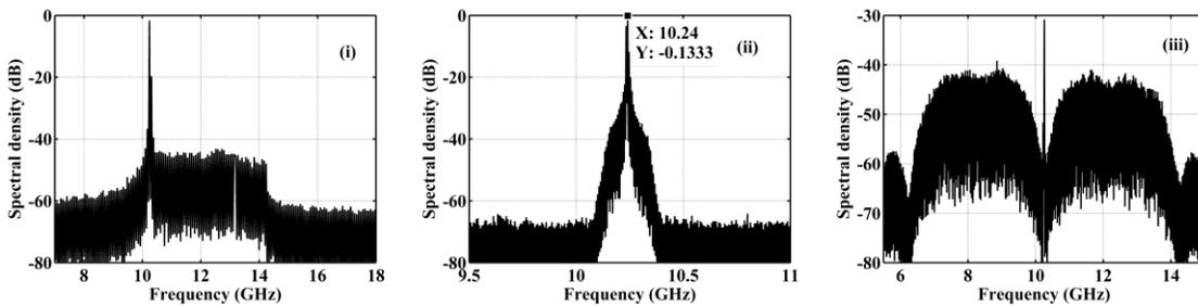
Fig. 2. RF spectra in downlink and uplink paths, measured after photodetector in BS (i), of the extracted carrier used in CU (ii), and uplink data (iii).
