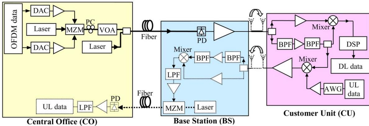
Fig. 1. Experimental setup for the mm-wave OFDM-RoF system. UL: up-link, DL: down-link, PC: polarization controller, VOA: variable optical attenuator, BPF: band-pass filter, LPF: low-pass filter, AWG: Arbitrary waveform generator, PD: Photo detector, MZM: Mach-Zehnder modulator. Dotted lines indicate functions not implemented in the experiment but needed for a full duplex system.
