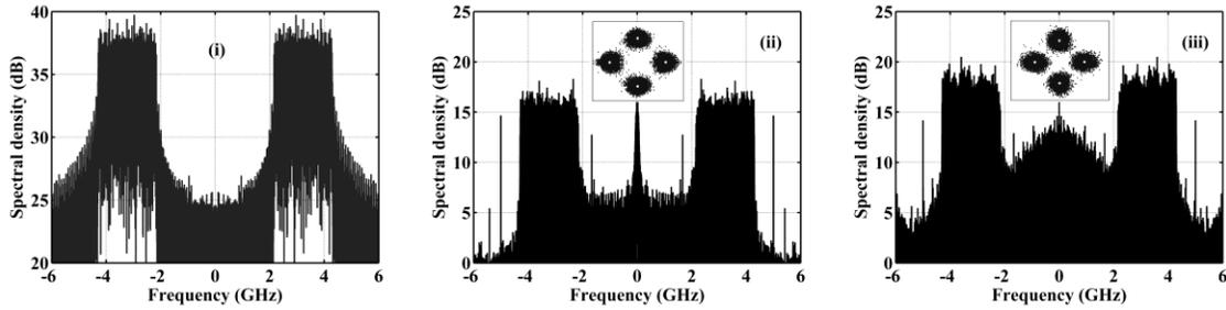
Fig. 3. OFDM spectra with 50% guard band, generated at the CO (i), measured at the CU using CER (ii) and measured at the CU using self-homodyne (iii). The insets in (ii) and (iii) show the respected received constellation diagrams.
