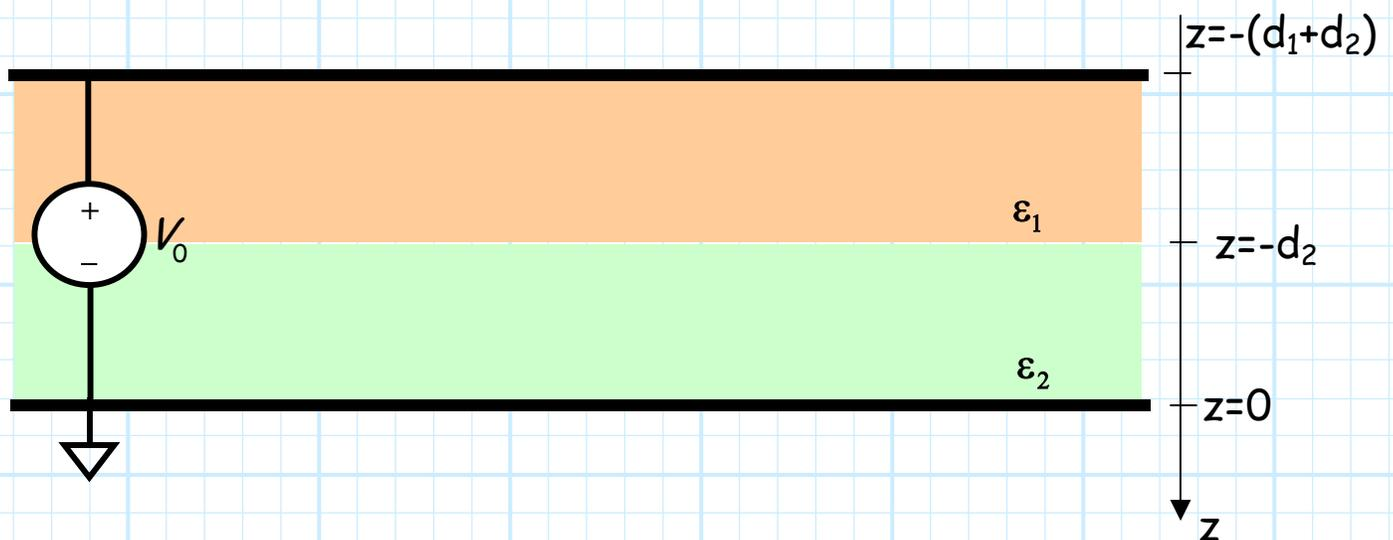
The **top** dielectric layer has thickness  $d_1$  and permittivity  $\epsilon_1$ , while the **bottom** layer has thickness  $d_2$  and permittivity  $\epsilon_2$ .
