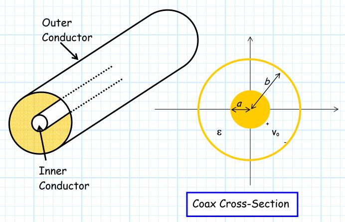
The coax has an outer diameter b, and an inner diameter a. The space between the conductors is filled with dielectric material of permittivity  $\epsilon$ .
