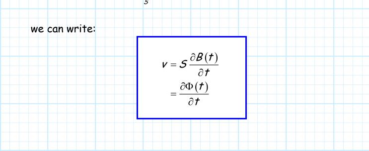
For this case, the **voltage** across the resistor is proportional to the **time derivative** of the **total magnetic flux** passing through the aperture formed by contour C.
