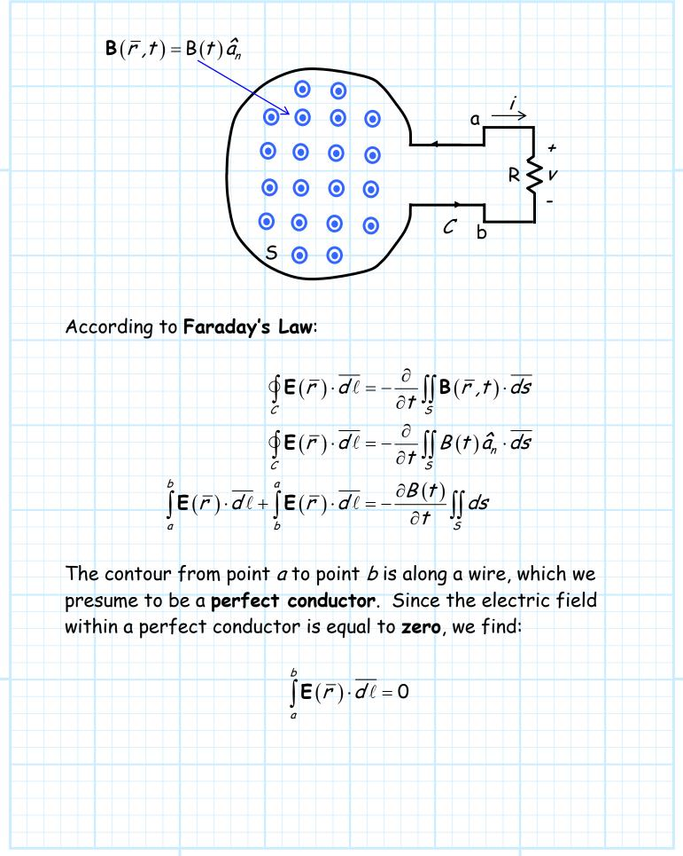
Likewise, if we integrate through the **resistor** from point *b* to point *a*, we find:
