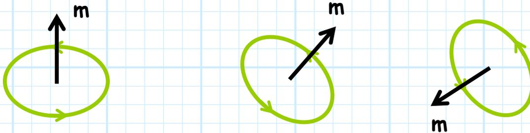
Note the direction is defined using the **right-hand rule** with respect to the direction of current  $I$ .
