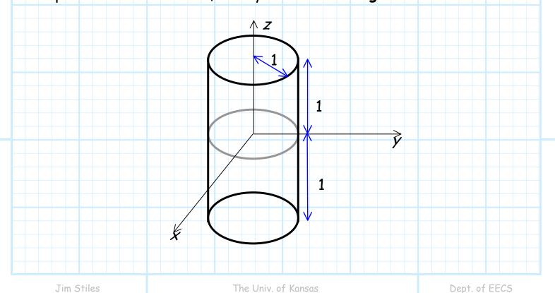
This is a **complex**, **closed** surface. We will define the **top** of the cylinder as surface  $S_1$ , the **side** as  $S_2$ , and the **bottom** as  $S_3$ . The surface integral will therefore be evaluated as:
