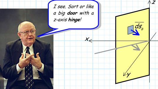
Note the differential surface vector  $\overline{ds_{\phi}}$  is **orthogonal** to this surface at every point.
