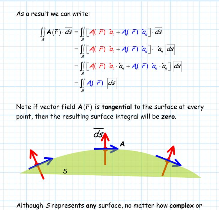
Although 5 represents any surface, no matter now complex or convoluted, we will study only basic surfaces. In other words,  $\overline{ds}$  will correspond to one of the differential surface vectors from Cartesian, cylindrical, or spherical coordinate systems.
