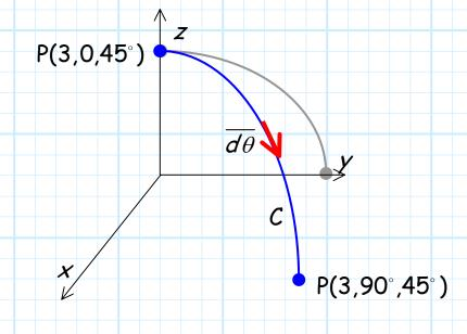
Finally, we could fix coordinates r and  $\theta$  and vary coordinate  $\phi$  only—but we **already** did this in cylindrical coordinates! We **again** find that a **circular arc** is generated, an arc that is parallel to the x-y plane.
