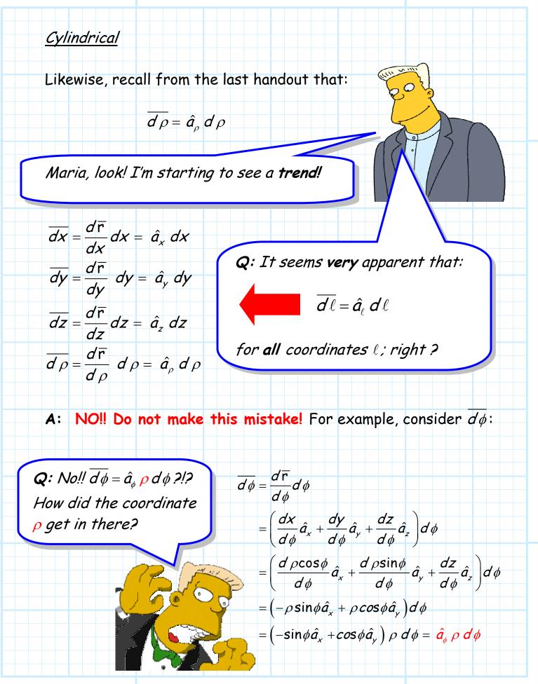
The scalar differential value  $\rho d\phi$  makes sense! The differential displacement vector is a directed distance, thus the units of its magnitude must be distance (e.g., meters, feet). The differential value  $d\phi$  has units of radians, but the differential value  $\rho d\phi$  does have units of distance.
