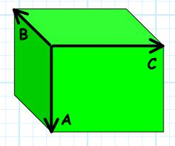
It is evident that the lengths of each side of the rectangular cube are  $|\mathbf{A}|$ ,  $|\mathbf{B}|$ , and  $|\mathbf{C}|$ , such that the **volume** of this rectangular cube can be expressed as:
