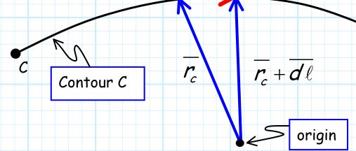
As a result, the differential line vector  $\overline{d\ell}$  is **always tangential** to every point of the contour. In other words, the direction of  $\overline{d\ell}$  always points "down" the contour.
