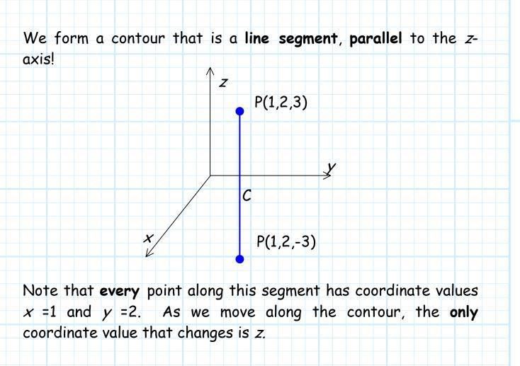
Therefore, the **differential** directed distance associated with a change in position from z to z + dz, is  $\overline{d\ell} = \overline{dz} = \hat{a}_z dz$ .
