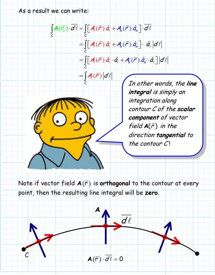
Although C represents any contour, no matter how complex or convoluted, we will study only basic contours. In other words,  $\overline{d\ell}$  will correspond to one of the differential line vectors we have previously determined for Cartesian, cylindrical, and spherical coordinate systems.
