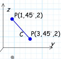
Note that **every** point along this segment has coordinate values  $\phi = 45^{\circ}$  and z = 2. As we move along the contour, the **only** coordinate value that changes is  $\rho$ .
