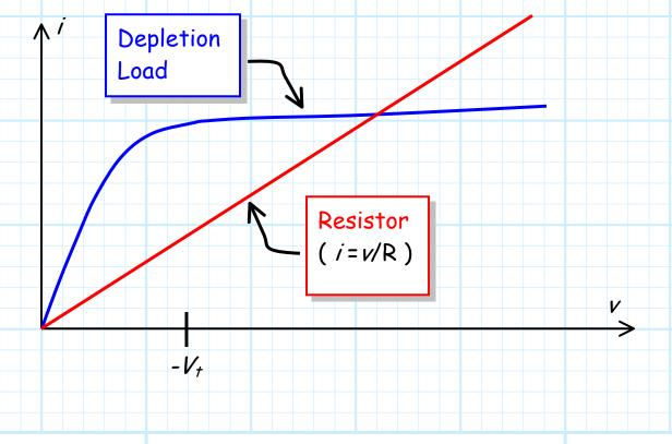
Note that the behavior of a Depletion Load and a resistor are very different—however they are precisely the same in two key ways:
