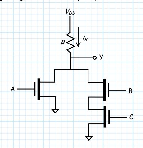
If the PDN is **open**, no current will flow ( $i_R = 0$ ), and thus there will be **no** voltage drop across the **Pull-Up Resistor** R—the output will be high, **just** like before!
