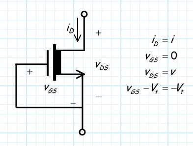
Q: But since  $v_{GS} = 0$ , isn't the NMOS device in cutoff?
