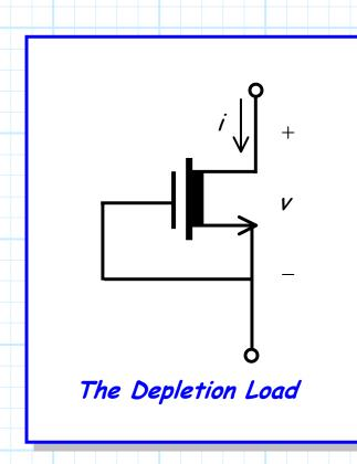
Since the depletion load is a two-terminal device, its behavior is defined by the relationship between the voltage vacross the device and the current i through it.
