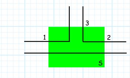
Since current is flowing **only** in these wires, the surface integral reduces to a surface integration over the cross section of **each** of the three wires:
