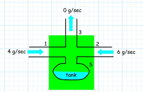
In addition to being a sink for water, this tank can also be a source. As a result, the current exiting pipe 3 could also exceed 10 gallons/second!
