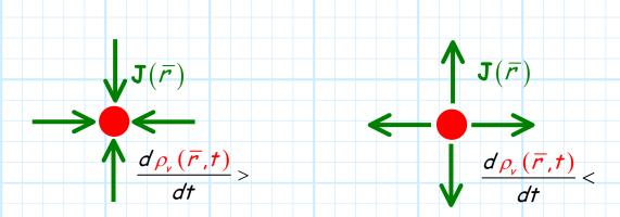
Current is **converging** on point, therefore charge density is **increasing**.
