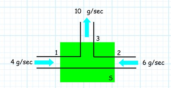
If a current of 4 gallons/second enters the node through pipe 1, and another 6 gallons/second enters through pipe 2, then 10 gallons/second must be leaving the node through pipe 3.
