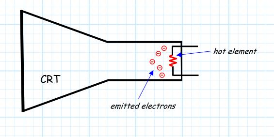
Then, an electric field  $\mathbf{E}(\bar{r})$  with large magnitude is created within the tube. The resulting force  $(\mathbf{F} = Q_e \mathbf{E}(\bar{r}))$  accelerates the electrons toward the front, creating a stream of electrons—a "cathode ray".
