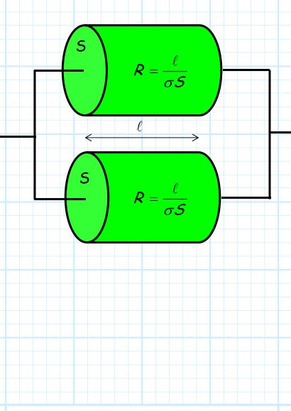
We can view this as a single resistor with a total cross sectional area of 2*.5.* Thus, its total resistance is:
