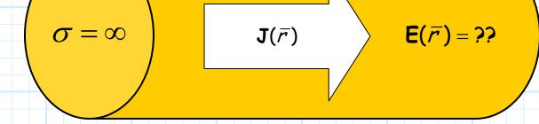
**Q:** What is the **electric field**  $\mathbf{E}(\overline{r})$  within this perfectly conducting material?
