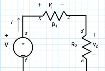
We find that if the **voltage source** is on (i.e.,  $V \neq 0$ ), then there will be electric potential differences (i.e., voltage) between different points of the circuit. This can **only** be true if **electric fields** are present!
