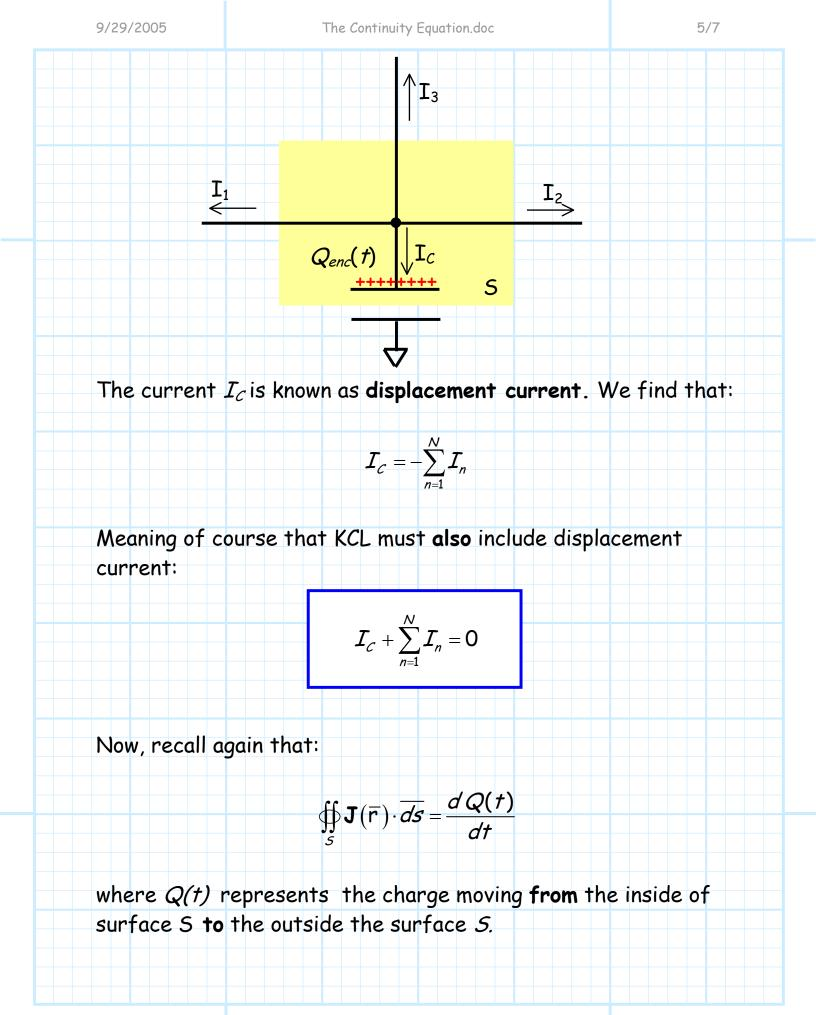
Note an increase in the charge **outside** the surface *S* results in a corresponding decrease in the total charge **enclosed** by *S*(i.e.,  $Q_{enc}(t)$ ). Therefore:
