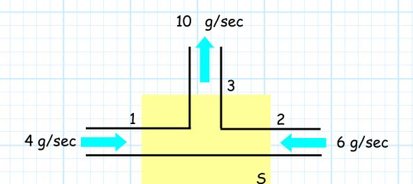
If a current of **4** gallons/second **enters** the node through pipe 1, and another **6** gallons/second **enters** through pipe 2, then **10** gallons/second **must** be **leaving** the node through pipe 3. The reason for this of course is that water cannot be **created** or **destroyed**, and therefore if water **enters** surface S at a rate of 10 gallons/sec, then water must also **leave** at the same rate.
