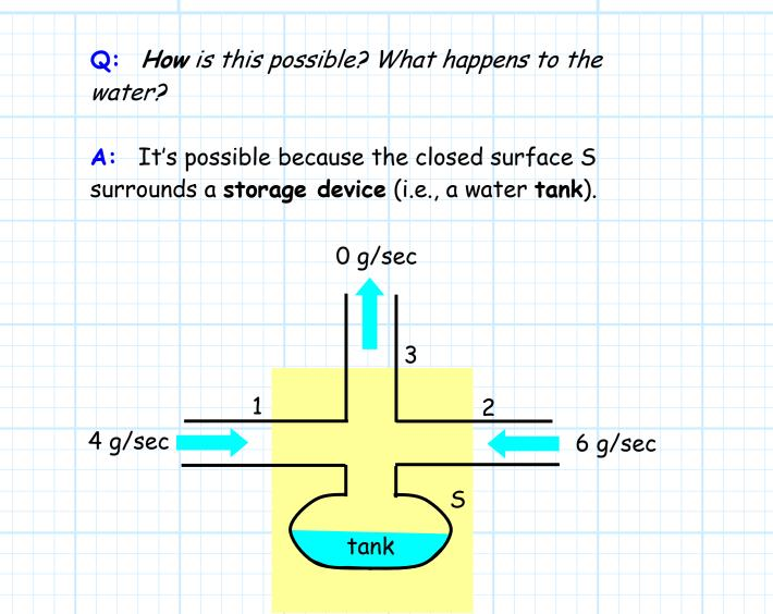
In addition to being a **sink** for water, this tank can also be a **source**. As a result, the current exiting pipe 3 could also **exceed** 10 gallons/second !
