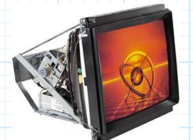
An almost perfect application of the Lorentz Force Law is the **Cathode Ray Tube** (CRT)—the device at the heart of every **television** and computer **monitor** (or, at least, the non-plasma/LED kind!).
