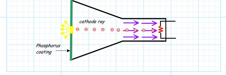
More specifically, the **spot** on the coating where the cathode ray strikes begins to glow (i.e., **fluoresces**). The **larger** the electric field, the higher the energy and thus the **brighter** the glow. Thus, we can **modulate** the light intensity by **changing** the electric field magnitude as a function of **time**.
