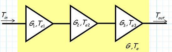
These three devices together can be thought of as **one** new microwave device.
