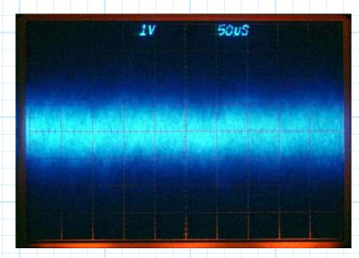
For example, consider the **frequency spectrum** of a noise process  $v_n(t)$ :
