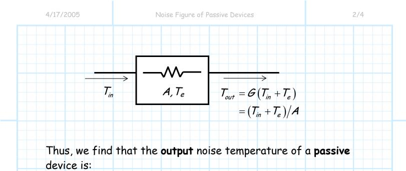
$$T_{out} = \mathcal{G}\left(T_{in} + T_{e}\right)$$
