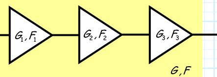
These three devices together can be thought of as **one** new microwave device.
