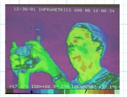
\* For objects on the Earth (i.e., terrestrial objects), the temperature is such that the emitted energy peaks in the infrared region.
