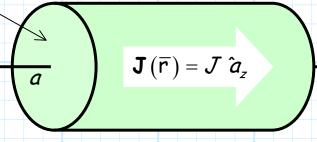
This cylinder is centered on the z-axis, and has length l. The surface area of the ends of the cylinder is S.
