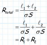
But, this result is not the **least bit** surprising, as the two resistors are connected in **series**!
