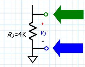
The electric potential at this point in the circuit is  $v_2$  volts greater than ground potential (i.e.,  $v_3$ ).
