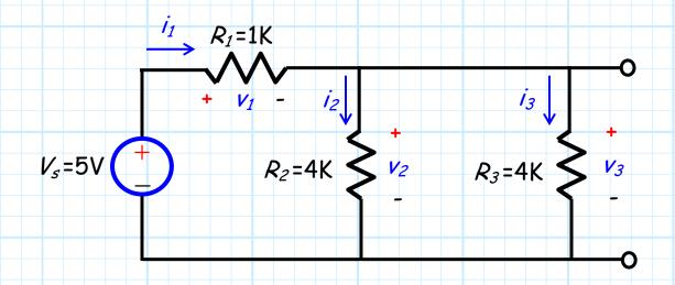
Note the voltage values in this circuit (i.e.,  $V_s$ ,  $v_1$ ,  $v_2$ ,  $v_3$ ) provide values of potential **difference** between two points in the circuit.
