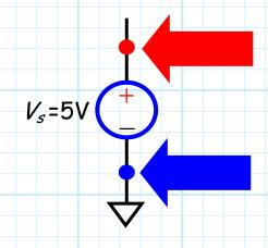
The electric potential at this point in the circuit is 5 volts greater than ground (i.e., 5 volts).
