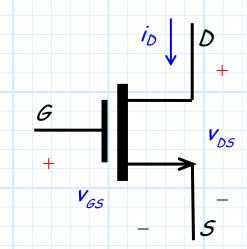
$$i_{D} = K \left[ 2 \left( v_{GS} - V_{t} \right) v_{DS} - v_{DS}^{2} \right]$$
