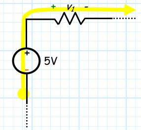
But, we could also use the convention that we subtract the circuit element voltage if we first encounter a plus (+) sign as we move along the loop, and add the circuit element voltage if we first encounter a minus (-) sign as we move along the loop!
