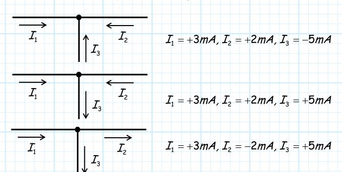
Remember, a **negative** value of current (or voltage) means that the current is flowing in the **opposite** direction (or polarity) of that denoted in the circuit.
