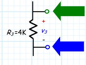
The electric potential at this point in the circuit is  $v_3$  volts greater than:
