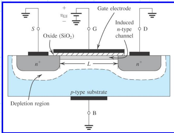
The electric field under the gate electrode will **repel** positively charged holes, but will **attract** negatively charged free electrons!
